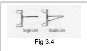
For pulls over 70% rated line pull, we recommend the use of the snatch block/pulley block to double line the wire rope. Fig 3.4
